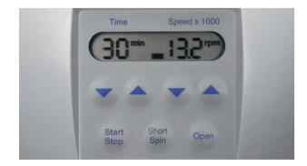
Use the arrow keys to easily select run time and speed
